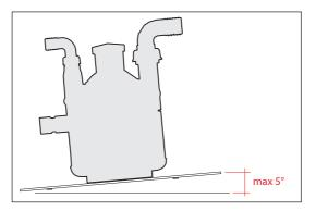
**Fix the pump** by screwing the pump support onto the base of the machine with suitable screws, tightening appropriately.
