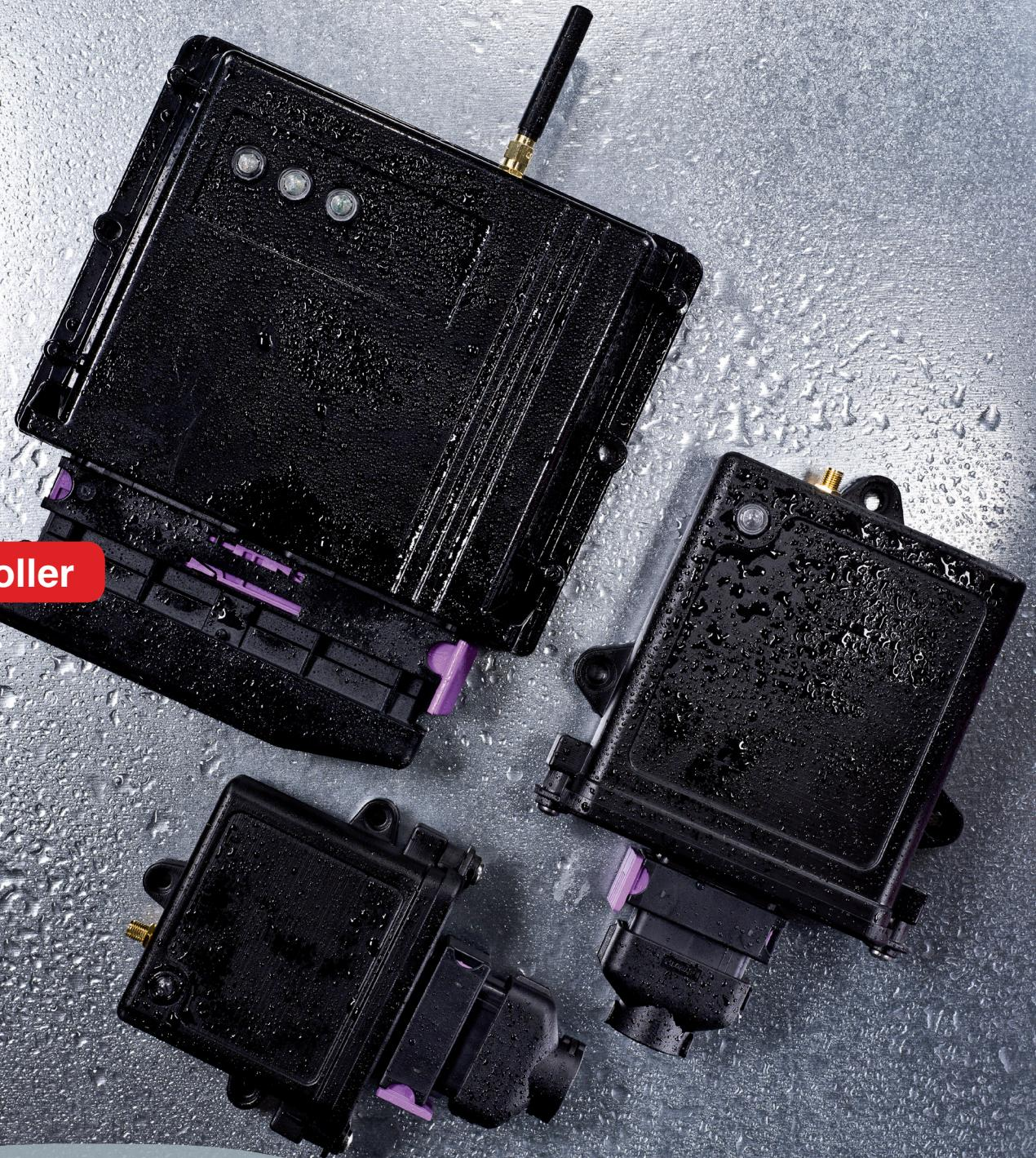
The Controller range with 8, 20 and 32 output,
