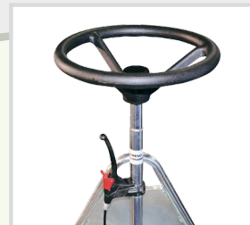
ERGONOMIC STEERING WHEEL AND PARKING BRAKE LEVER
