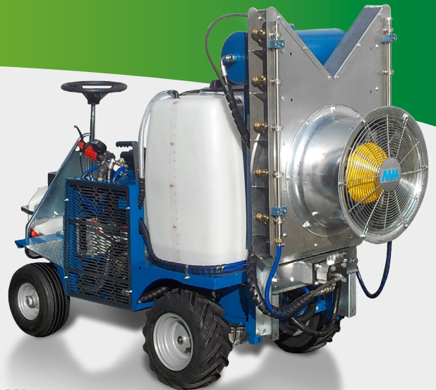
VERSION WITH LINEAR FAN FOR TREATMENTS BETWEEN THE ROWS
